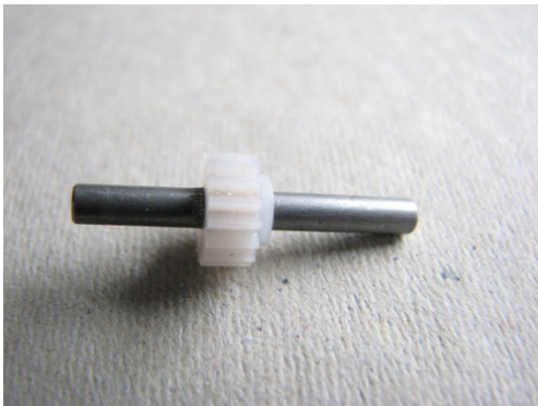
Gear on new axle – note boss faces chassis centre.
