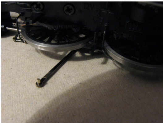
Rod placed over rivet.
